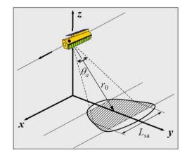
azimuth resolution = half antenna length in azimuth
