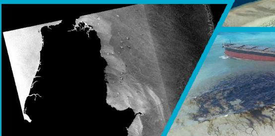
Detection and monitoring of oil-like features in the coastal ocean using Sentinel-1 SAR and a fusion of machine learning and empirical methods
