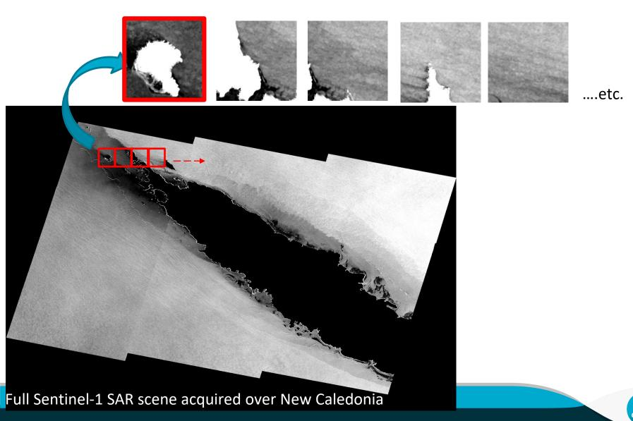
10 | Detection and monitoring of oil-like features in the coastal ocean using Sentinel-1 SAR and machine learning + empirical methods
